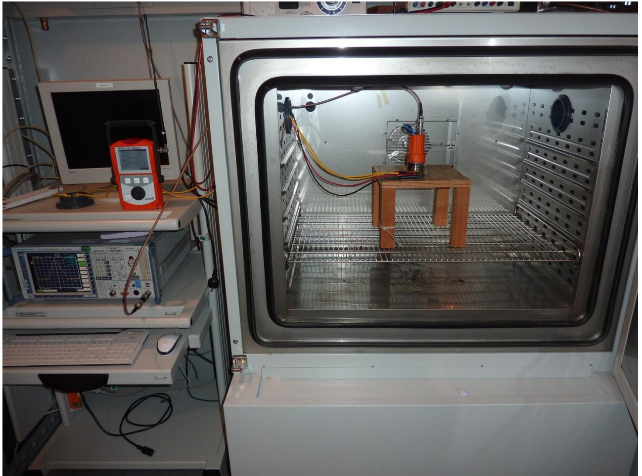
161191_04.JPG: Test setup – Temperature chamber
