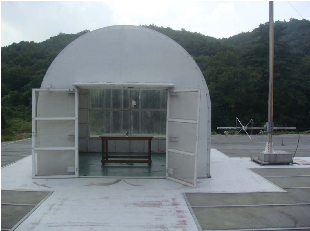
Radiated emission test below 1 GHz
