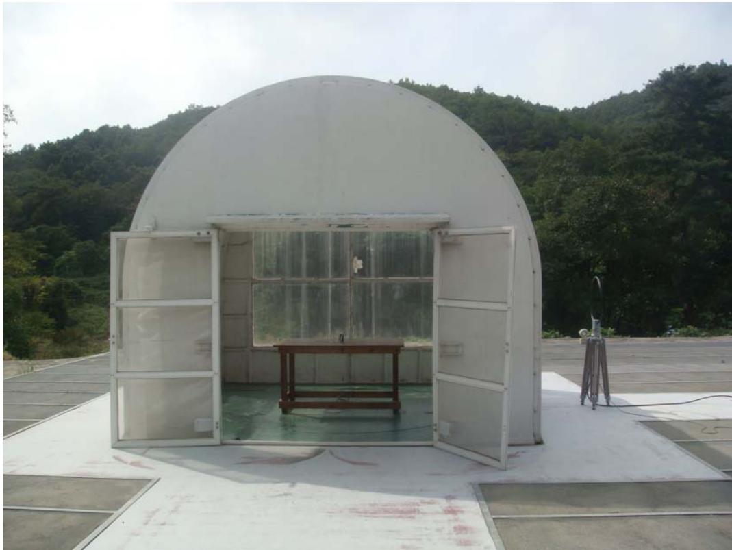
Radiated emission test below 1 GHz
