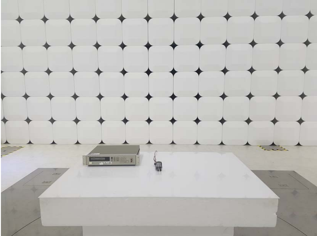
Radiated emissions - rear view
