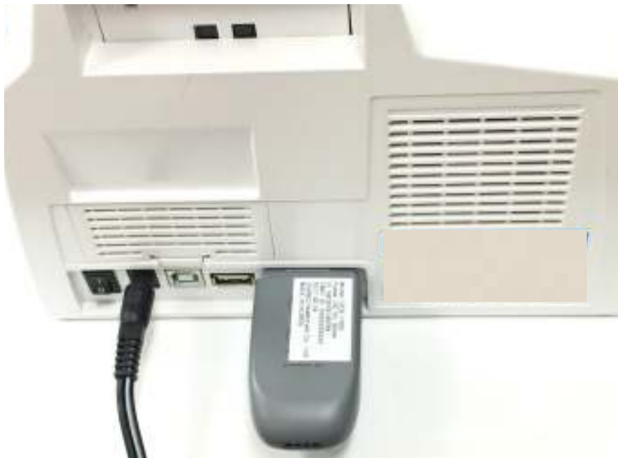
Figure 8. Oh' Care Bridge connected state.
