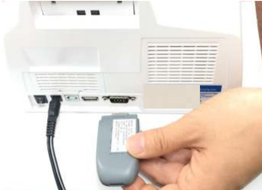
Figure 7 . Oh'Care Bridge on D-Sub 9
