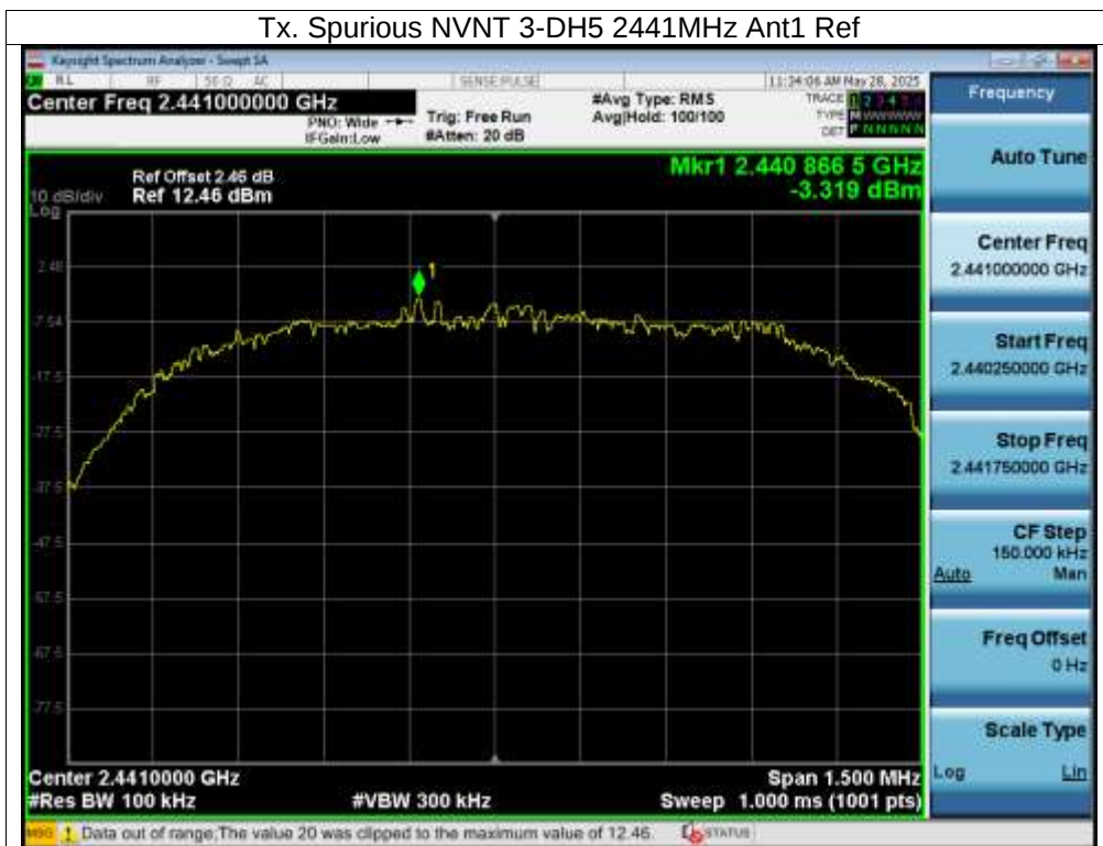
Tx. Spurious NVNT 3-DH5 2441MHz Ant1 Emission
