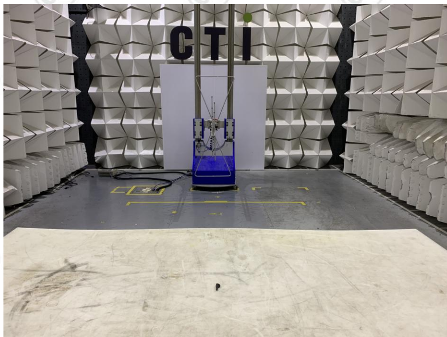
Radiated spurious emission Test Setup-1 right ear(Below 1GHz)
