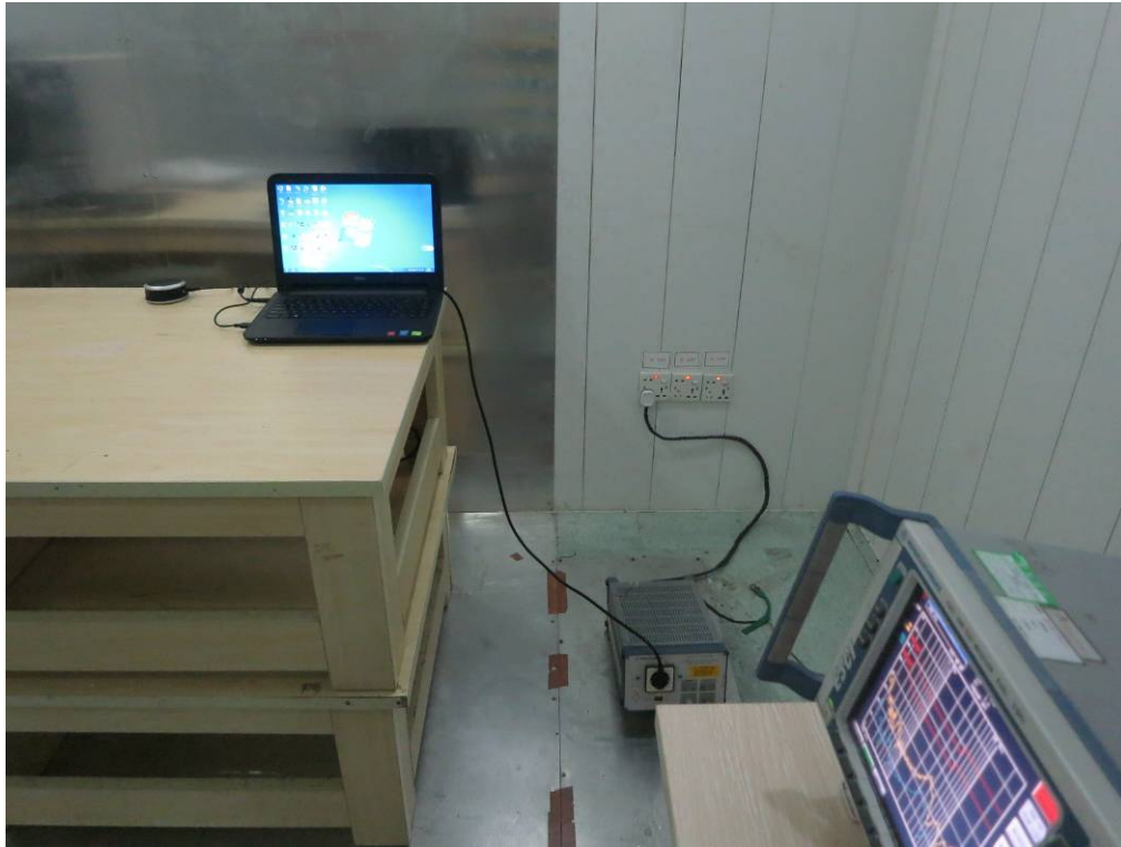
FCC RADIATED EMISSION TEST SETUP
