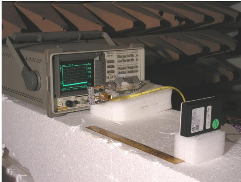
Figure 4: Radiated Emissions Test Setup Photograph(s).
