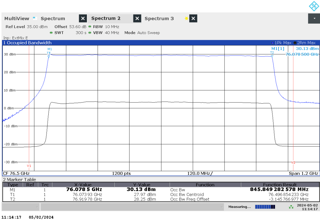
Plot no. 3: Peak Power EIRP, Peak detector, 10 MHz RBW due to pulse desensitisation.
