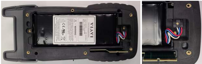
Figure B-6 Battery Cables and Release Clip
