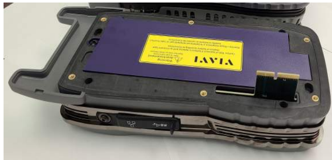
Figure B-3 Base Unit - RF Module Removed
