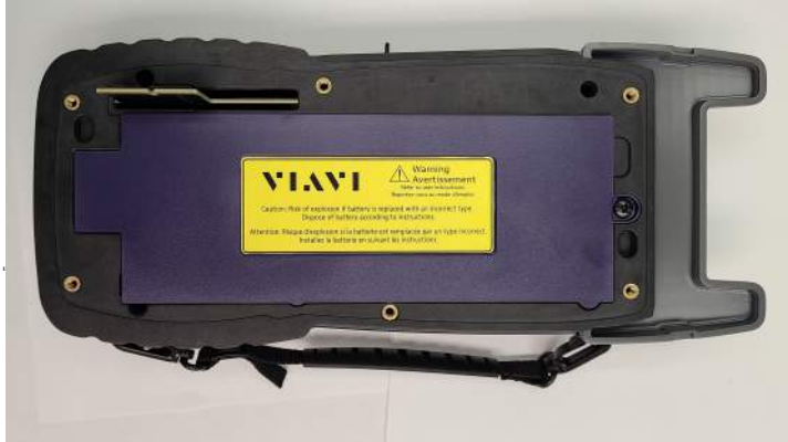
Figure B-5 Battery Cover Screw Location
