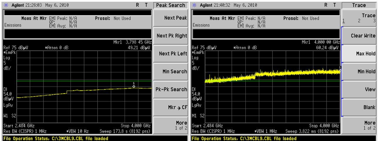
Average limit is 54 dBuV/m, Peak limit is 74dBuV/m
