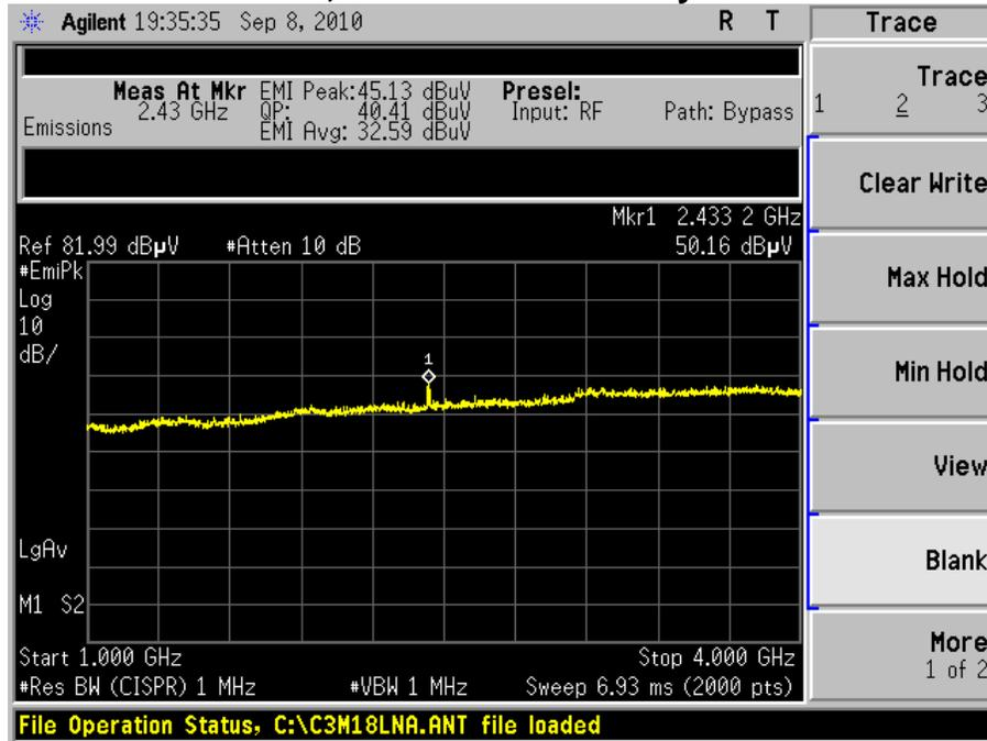
**Channel 11, Antenna Horizontally Polarized**
