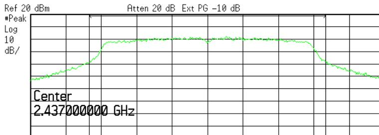
Center 2.437 GHz Span 30 MHz
