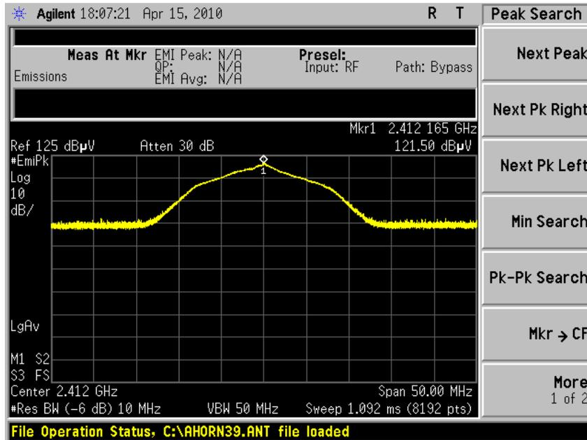
**Channel 11, Antenna Vertically Polarized, 2484.0-2500 MHz, at 3m**
