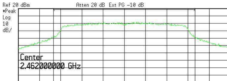
Center 2.462 GHz Span 30 MHz
