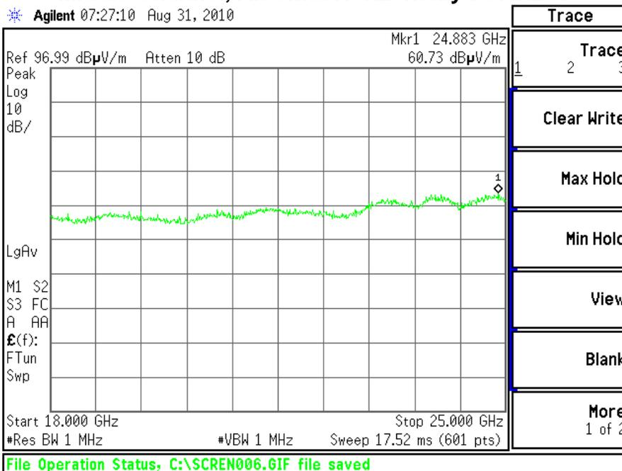
**Middle Channel, Antenna Horizontally Polarized**
