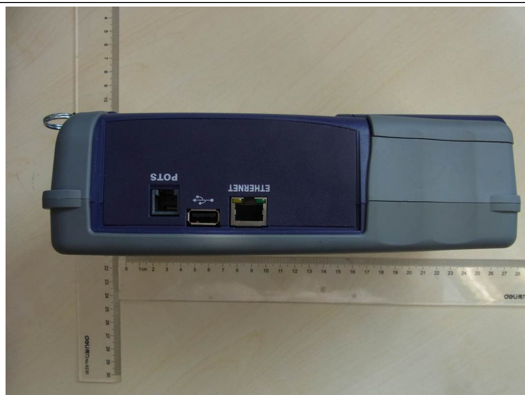
Figure 5: Side view SCTPS-AB-CU
