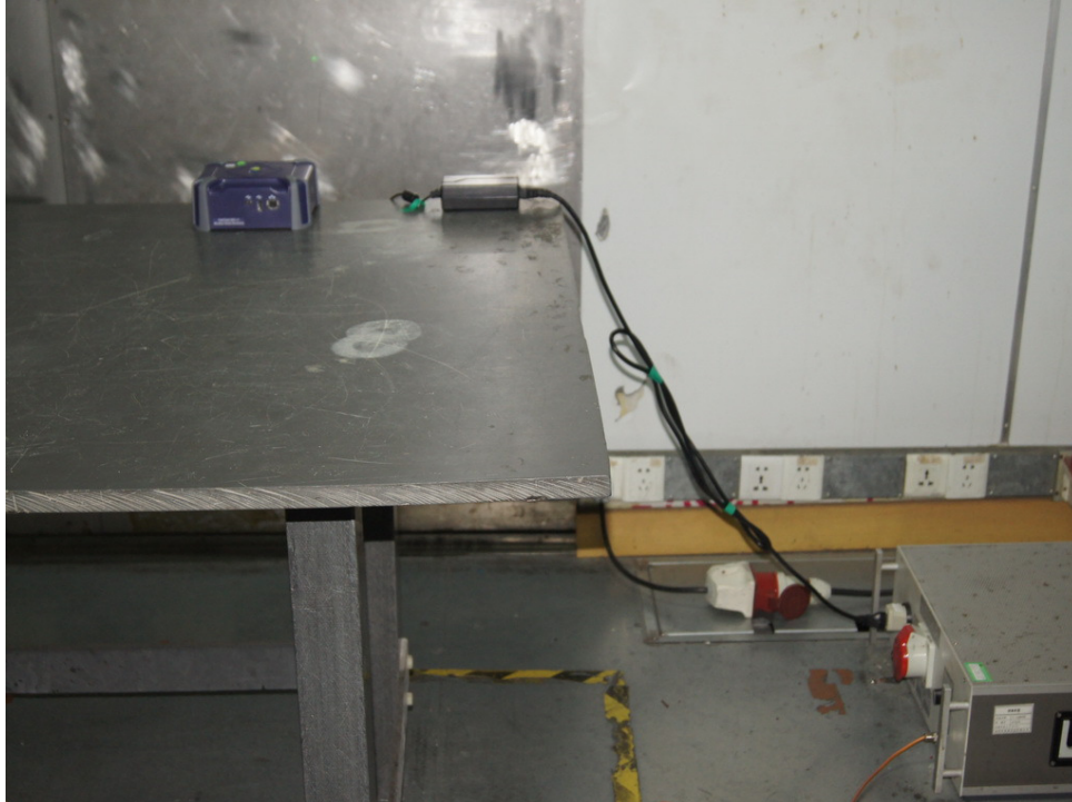
Photograph 7: Set-up for Conducted emissions
