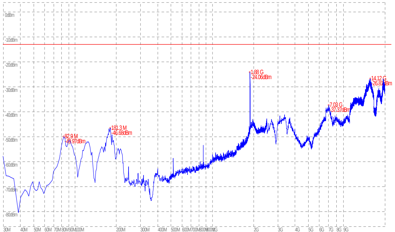
(Plot B.3: GSM 1900MHz Channel = 661, Test Antenna Horizontal)
