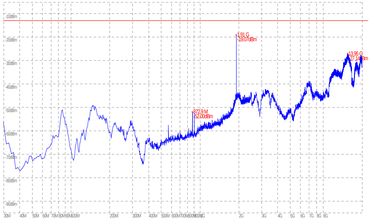
(Plot D.5: EGPRS 1900MHz Channel = 810, Test Antenna Horizontal)
