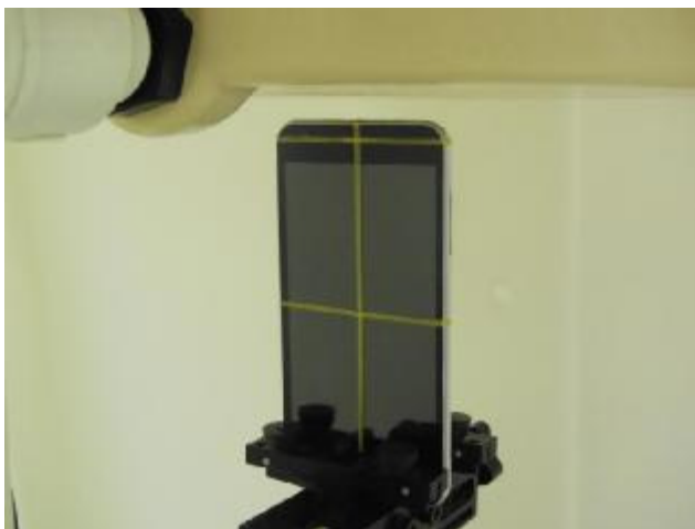
Top Side, Test Separation 10 mm
