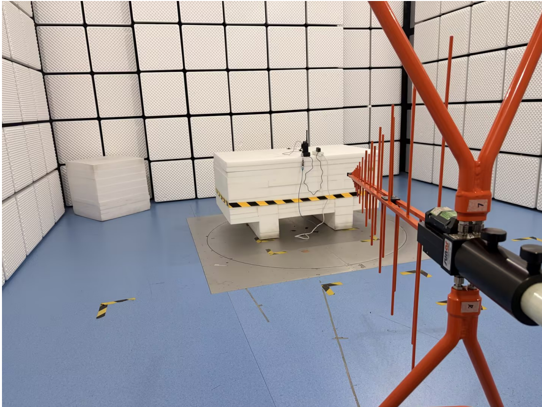
Radiation Emission - Back View (Below 1GHz) – For Charger
