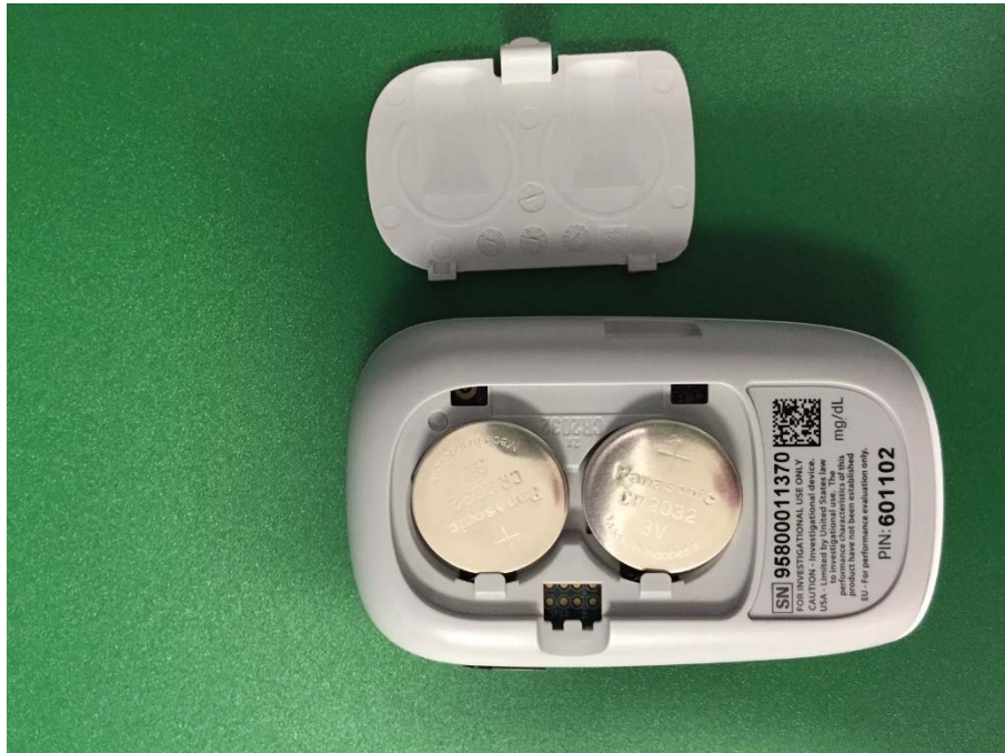
Photo 1: Battery cover removed
