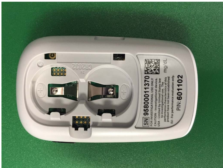
Photo 2: Battery cover removed
