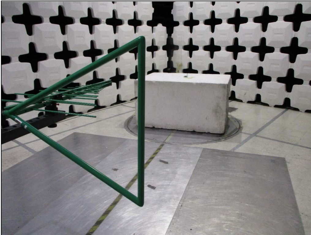
Test Setup for Spurious Radiated Emissions, 30-1000MHz – Antenna Polarization Horizontal
