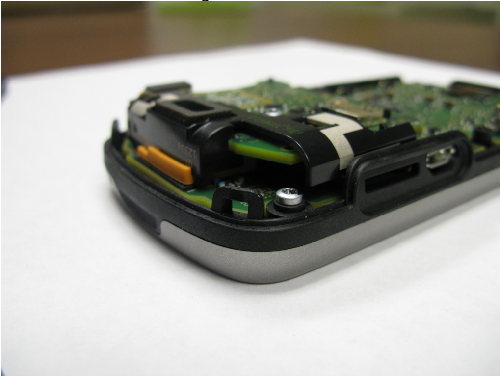
Bottom of Meter showing COMMS Board above Mother Board
