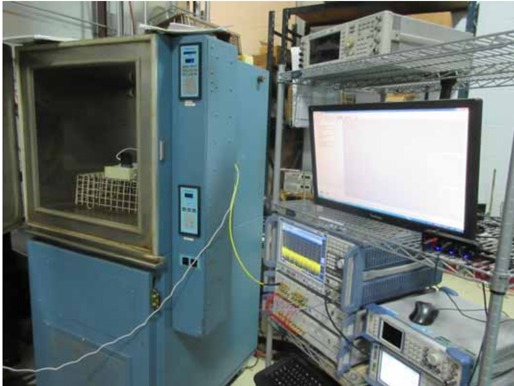
Test Setup for Antenna Conducted Emissions Tests
