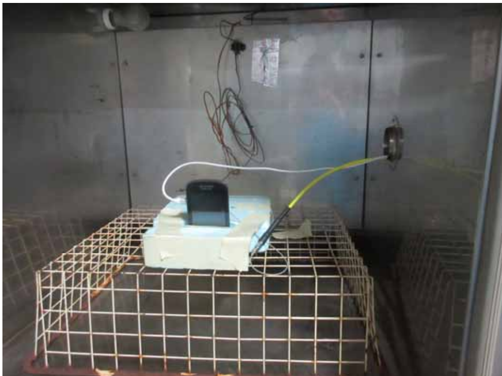
Test Setup for Antenna Conducted Emissions Tests
