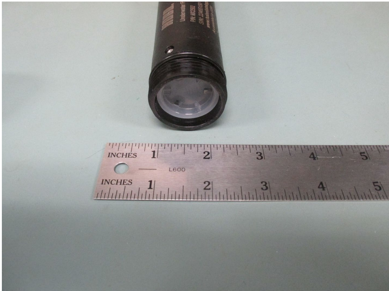
Left side view of clear plastic end cap which allows the user to see the status LED.
