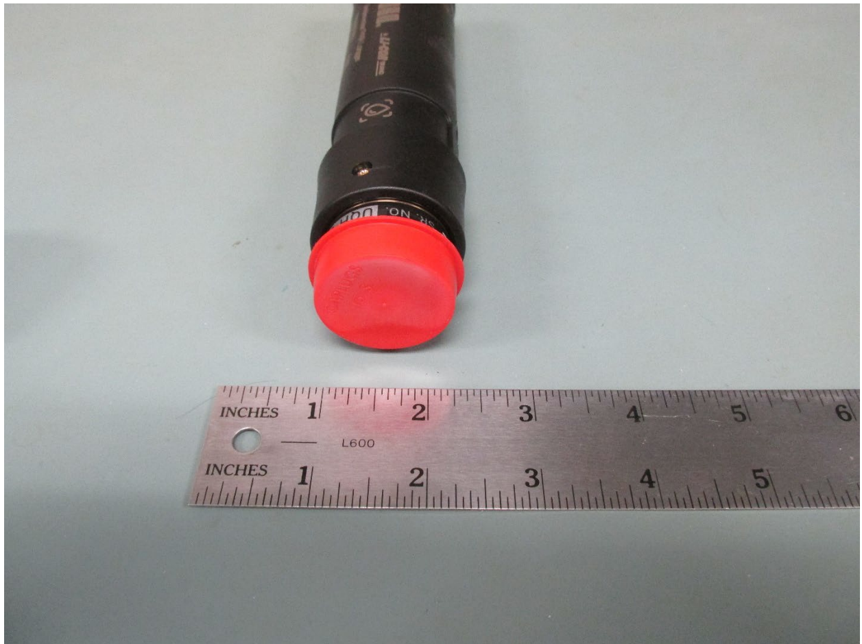
Right side view with red plastic protective cover over the PAR sensor.
