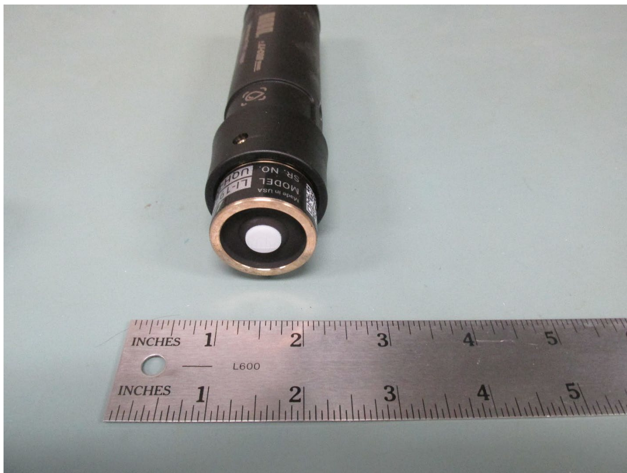
Right side view with red plastic protective cover removed, thus exposing the PAR sensor diffuser.
