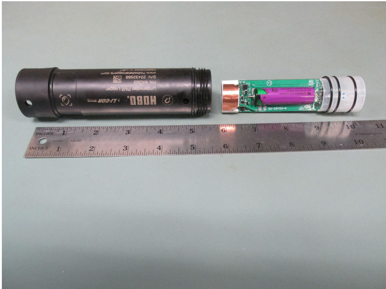
Logger inner assembly, position to slide into the plastic enclosure 85-29750.
