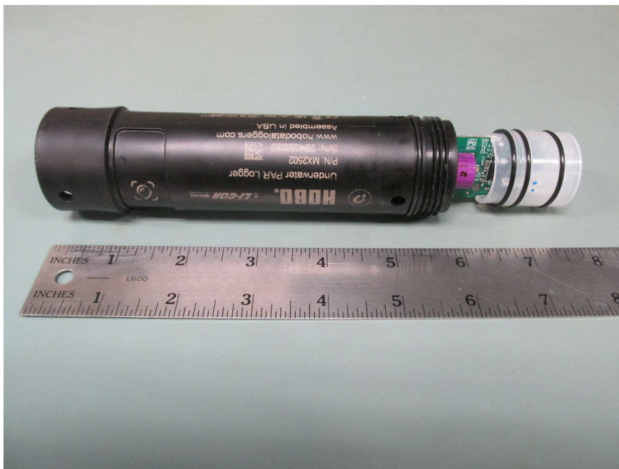
Logger inner assembly, partially slid into the plastic enclosure.
