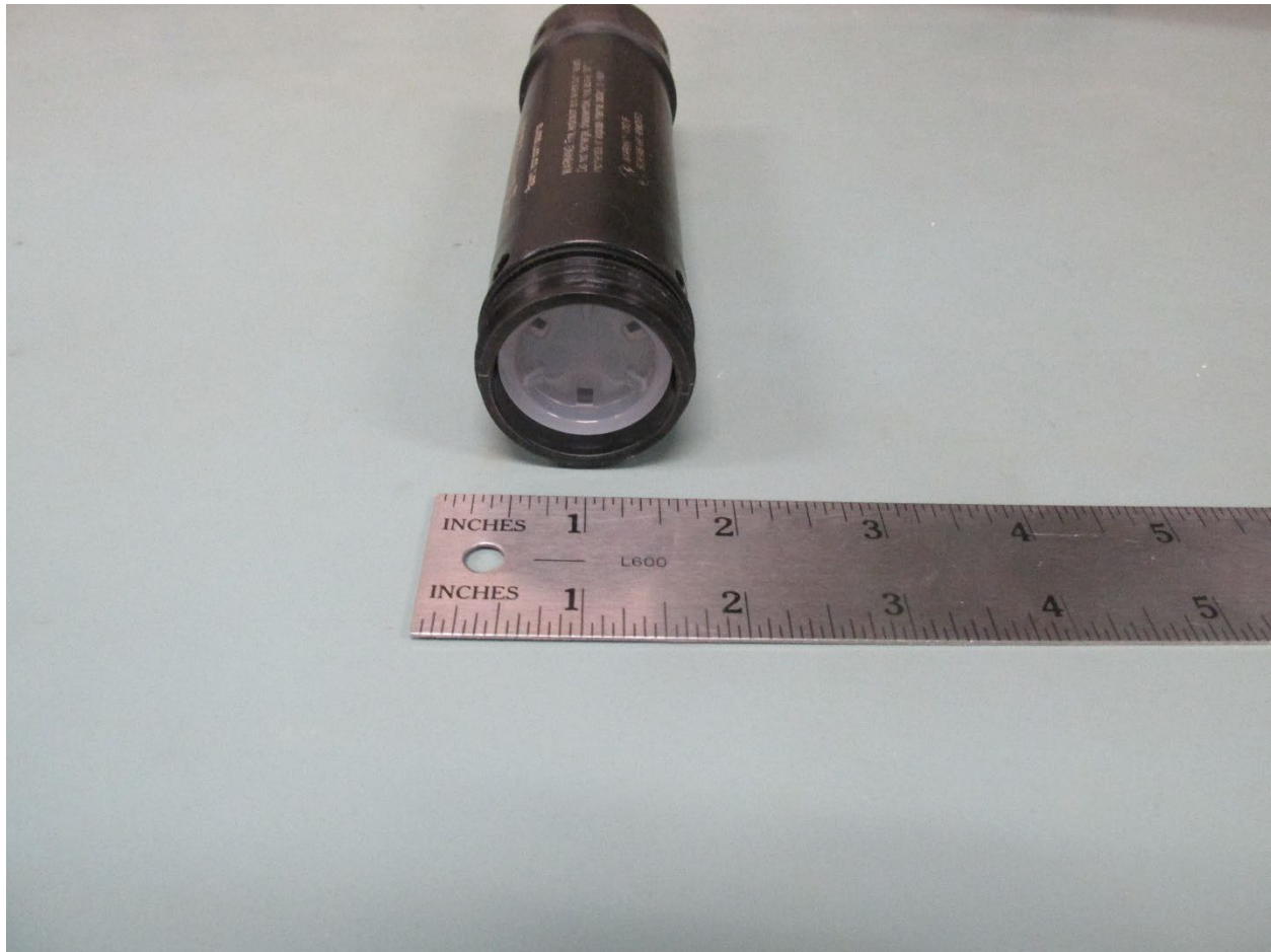
Logger inner assembly, fully slid into the enclosure, clear endcap side.
