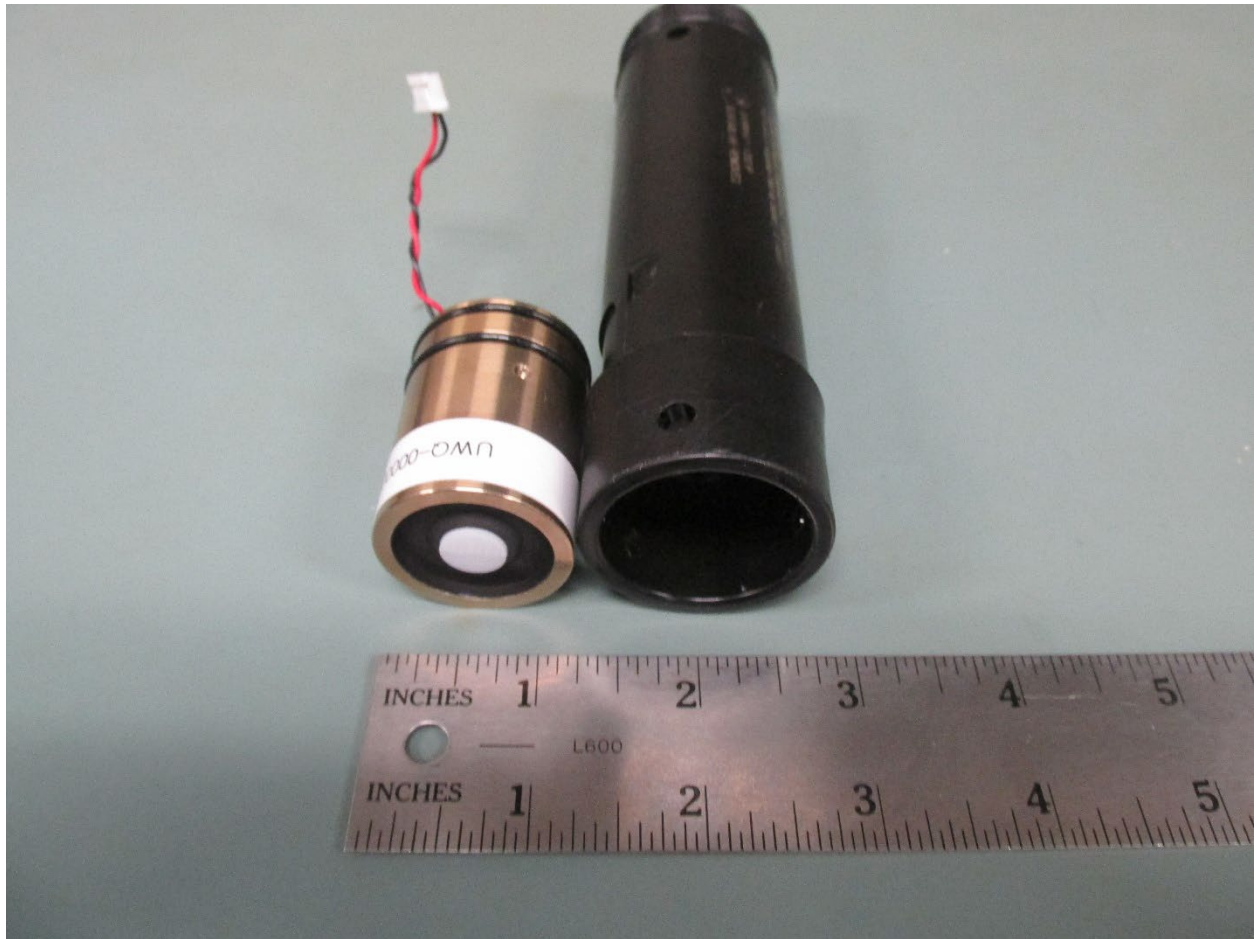
PAR light sensor assembly, front view, also showing where it will slide into the enclosure.
