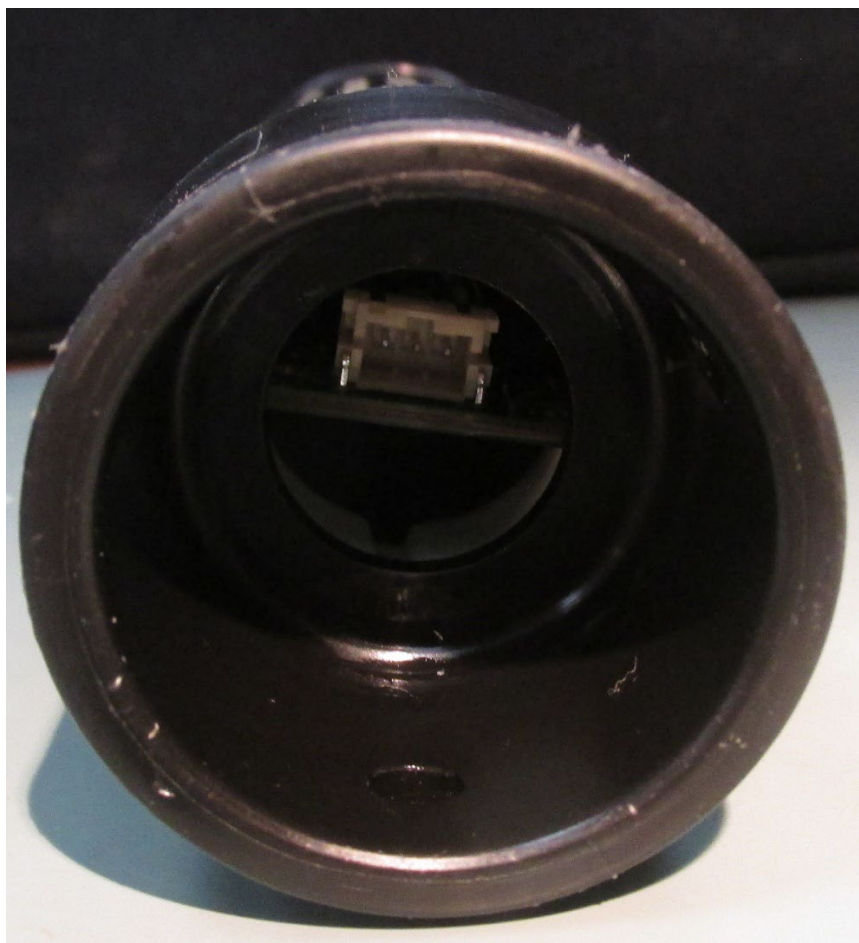
Logger inner assembly, fully slid into the enclosure, sensor side view.
