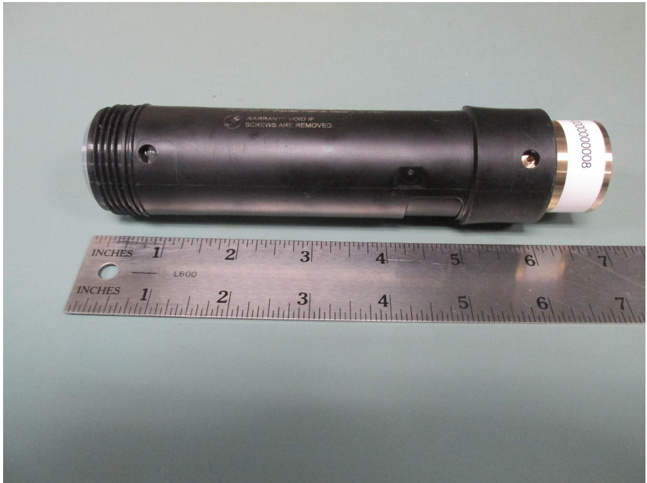
PAR light sensor assembly, slid into the enclosure.
