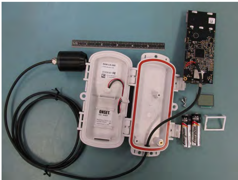
RXW-LIA-900 Exploded View with Sensor
