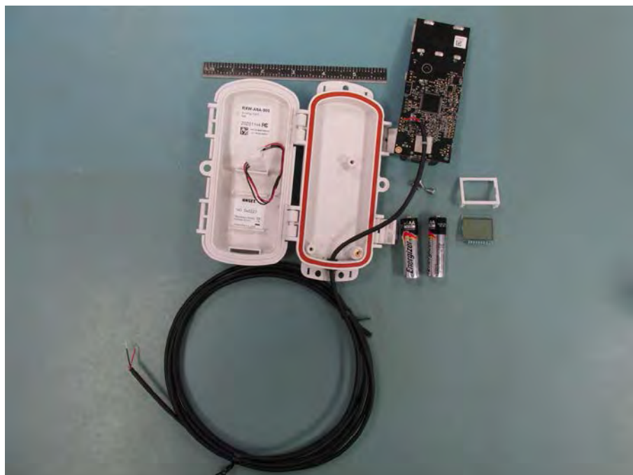
RXW-ANA-900 Exploded View with Sensor
