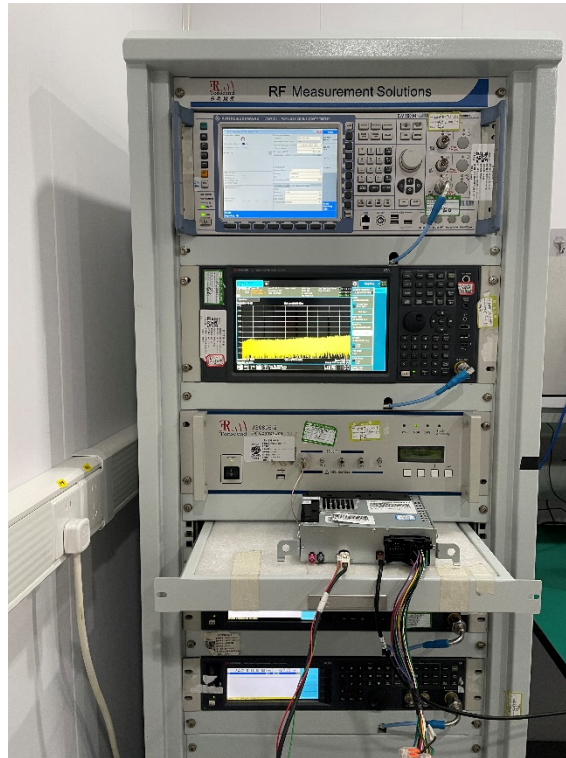
Description: Conducted Test Setup
