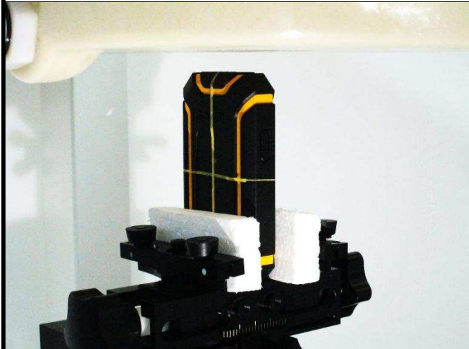
Top Side of EUT with 1.0 cm Gap
