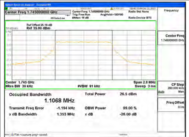
B66 / 1.4MHz / 256QAM/ Mid CH
