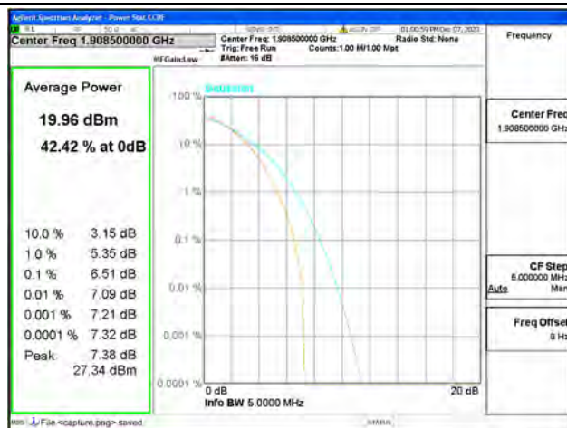
B2 / 3MHz / High CH / 64QAM
