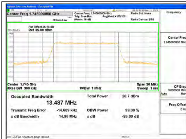
B66 / 15MHz / 64QAM/ Mid CH
