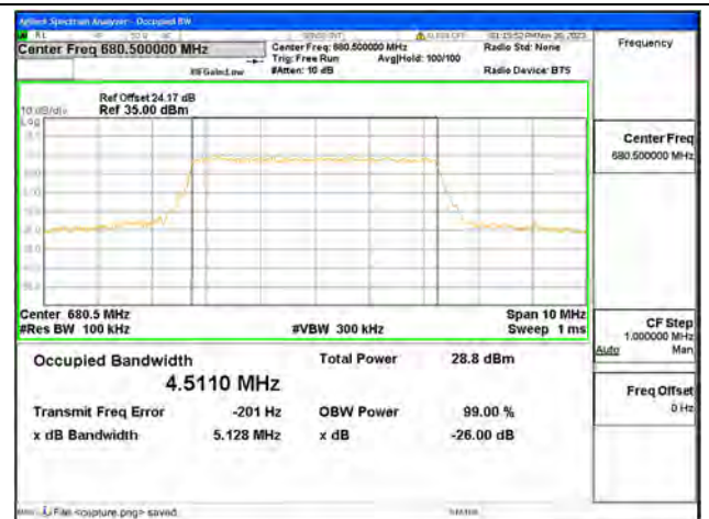
B71 / 5MHz / 16QAM/ Mid CH
