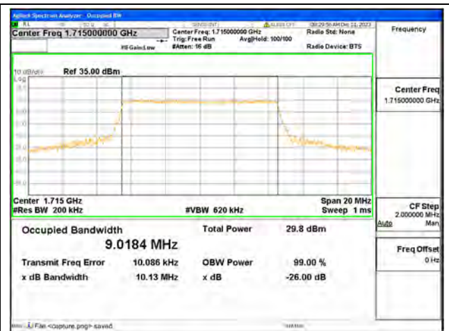
B66 / 10MHz / 16QAM/ Low CH
