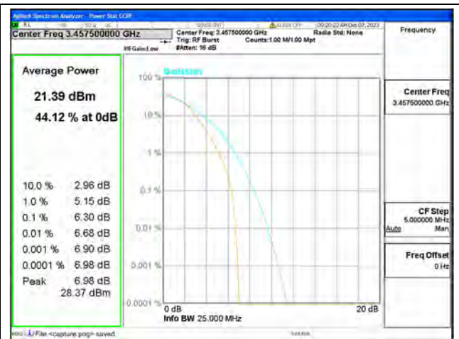
B42 / 15MHz / Low CH / 16QAM
