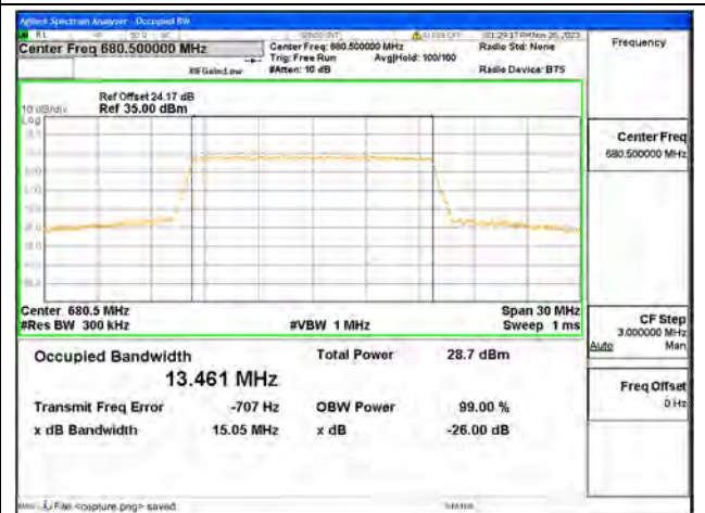
B71 / 15MHz / 16QAM/ Mid CH
