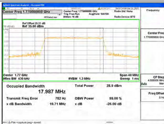
B66 / 20MHz / 64QAM/ High CH
