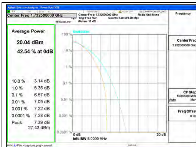
B4 / 3MHz / Mid CH / 64QAM
