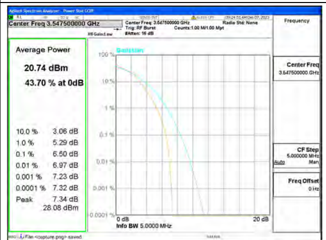
B42 / 5MHz / High CH / 16QAM
