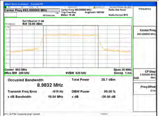
B71 / 10MHz / 16QAM/ High CH
