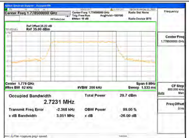
B66 / 3MHz / 16QAM/ High CH
