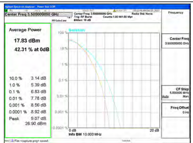
B42 / 10MHz / Mid CH / 256QAM
