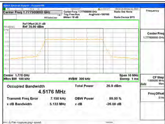
B66 / 5MHz / 256QAM/ High CH
