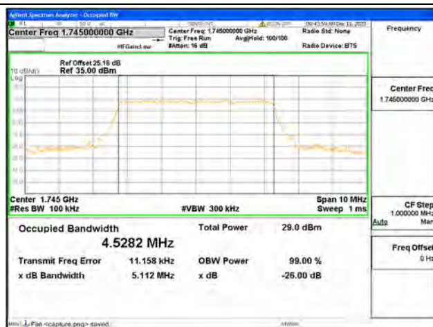
B66 / 5MHz / 64QAM/ Mid CH
