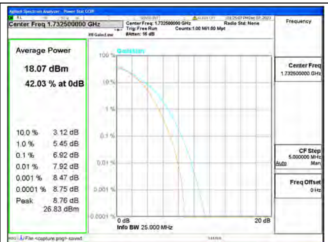
B4 / 15MHz / Mid CH / 256QAM
