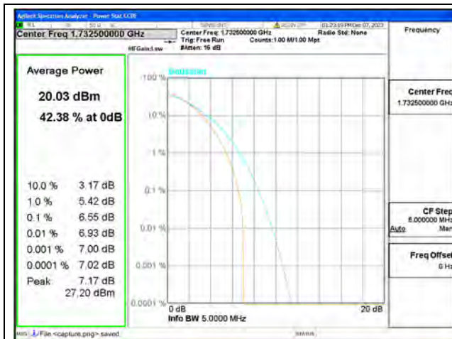
B4 / 1.4MHz / Mid CH / 64QAM
