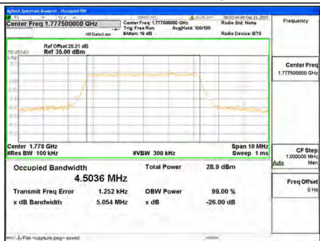
B66 / 5MHz / 64QAM/ High CH
