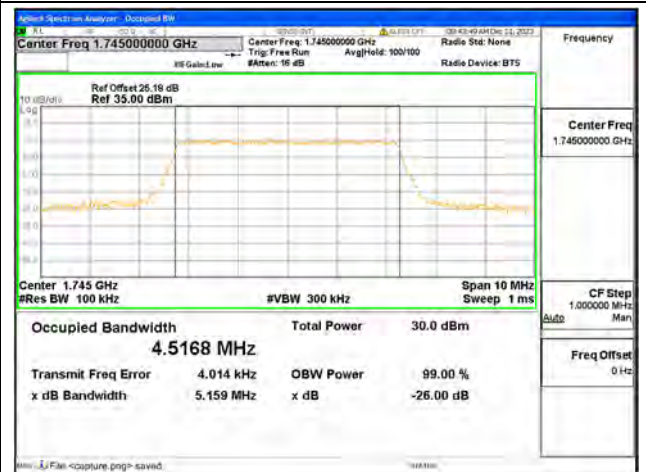
B66 / 5MHz / 16QAM/ Mid CH
