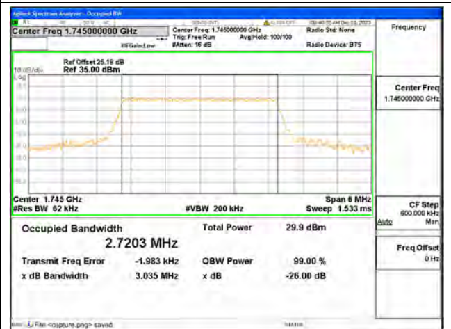
B66 / 3MHz / 16QAM/ Mid CH
