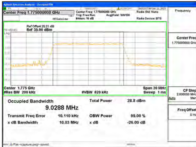
B66 / 10MHz / 64QAM/ High CH
