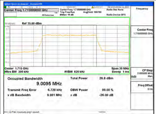
B66 / 10MHz / 256QAM/ Low CH
