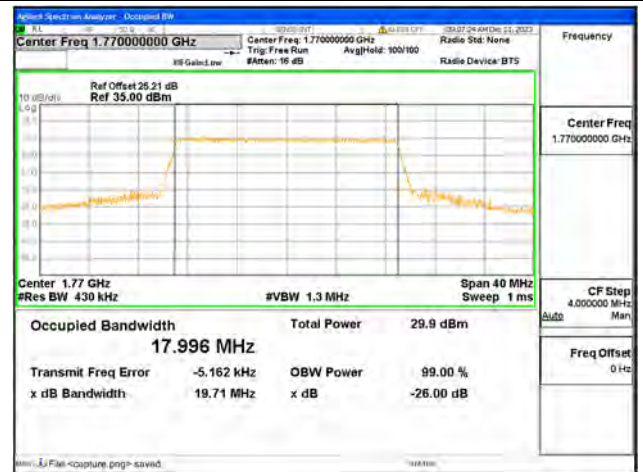
B66 / 20MHz / 16QAM/ High CH
