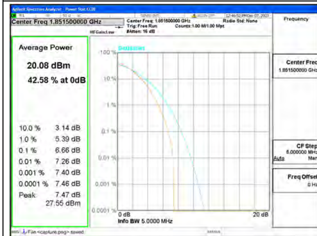
B2 / 3MHz / Low CH / 64QAM
