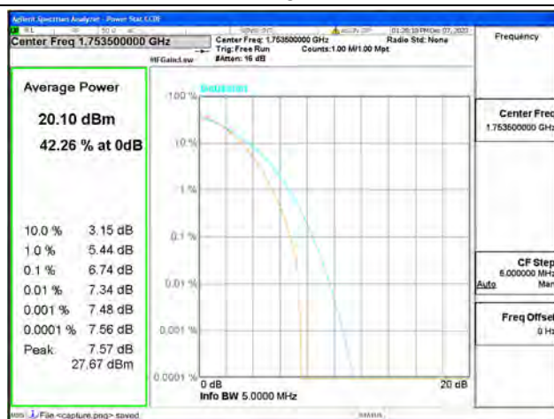
B4 / 3MHz / High CH / 64QAM
