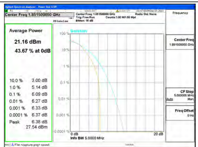
B25 / 3MHz / Low CH / 16QAM
