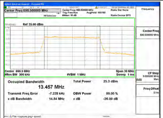
B71 / 15MHz / 256QAM/ High CH
