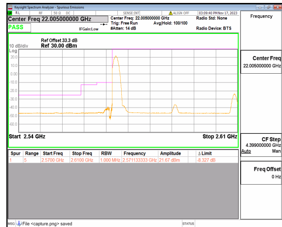
n38 40M DFT-s-OFDM QPSK Edge_1RB_Left Low
