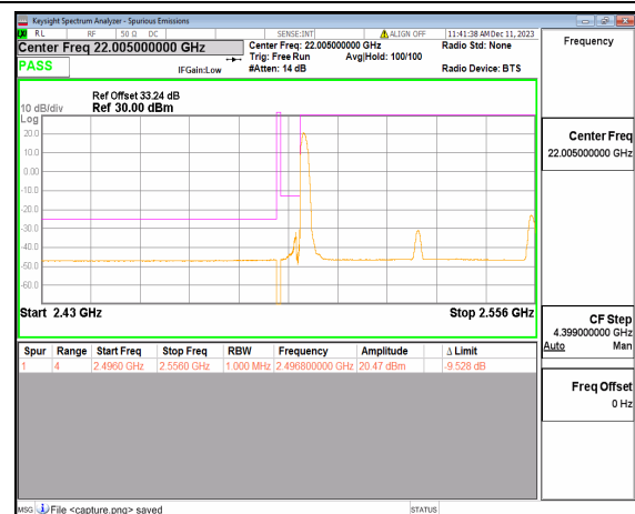
n41 60M DFT-s-OFDM QPSK Edge_1RB_Left Low
