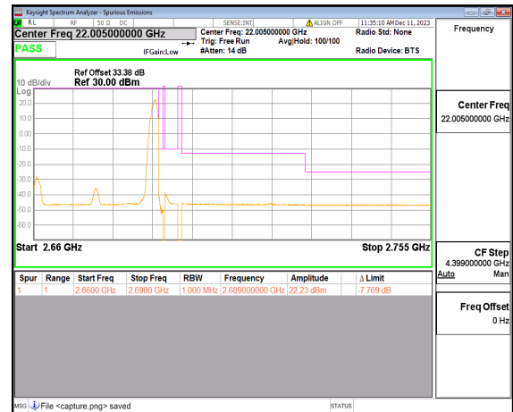
n41 30M DFT-s-OFDM QPSK Edge_1RB_Right High
