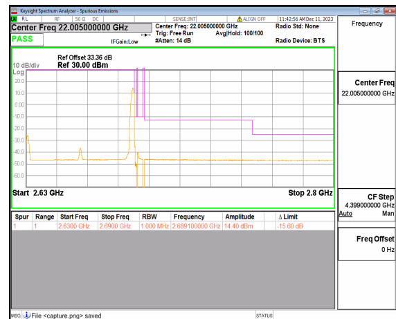
n41 60M DFT-s-OFDM QPSK Edge_1RB_Right High
