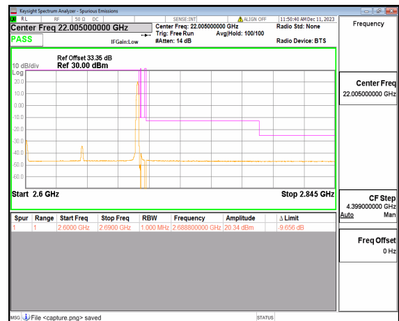
n41 90M DFT-s-OFDM QPSK Edge_1RB_Right High
