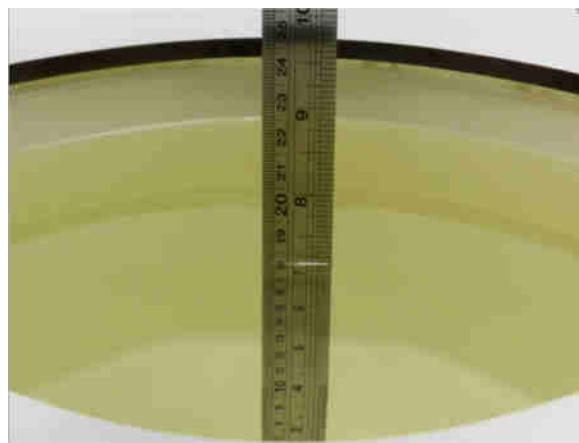
Fig 11.2 Photo of Liquid Height for Body SAR
