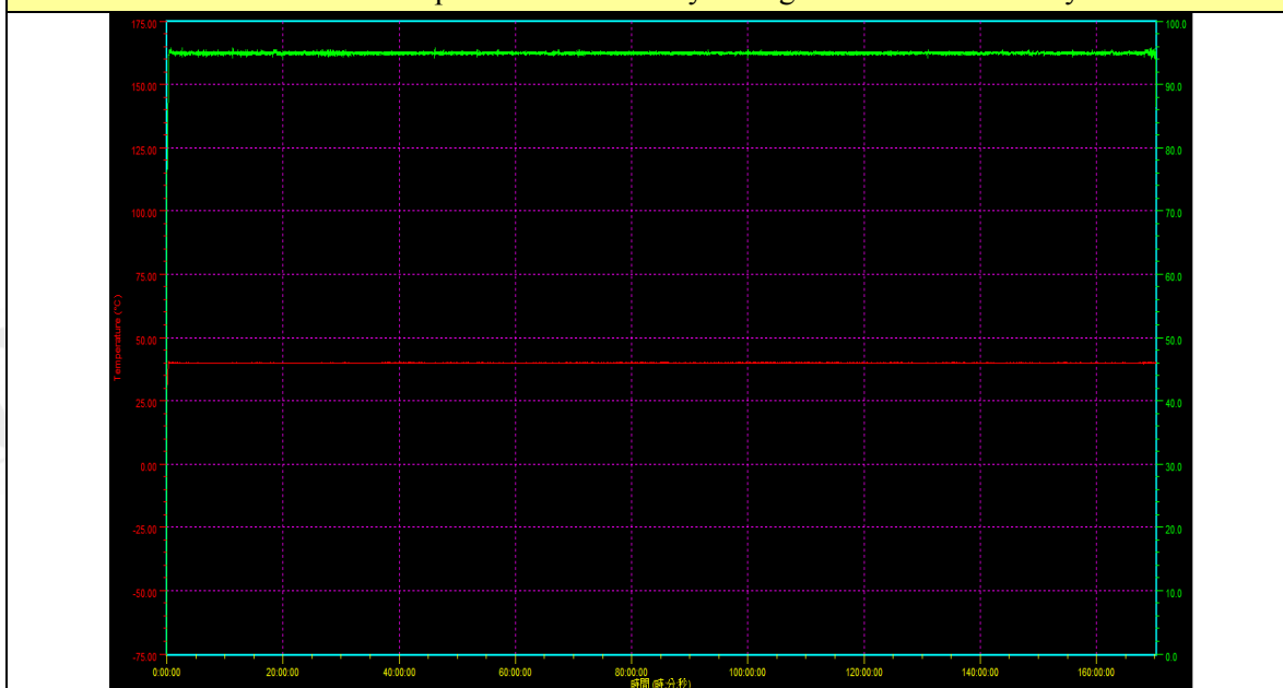
11. Salt Mist Temperature & Humidity Storage Test Profile --2 ND cycle
