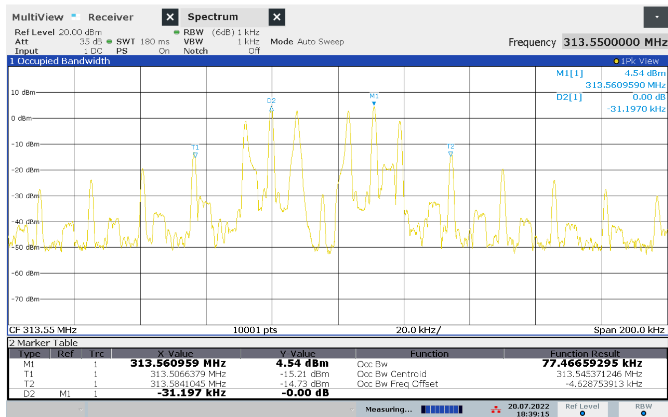
Figure 2-15 – Occupied Bandwidth – 313.55 MHz
