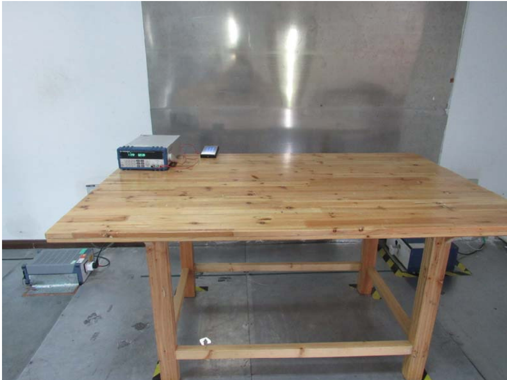
Conducted Emissions Setup Front View
