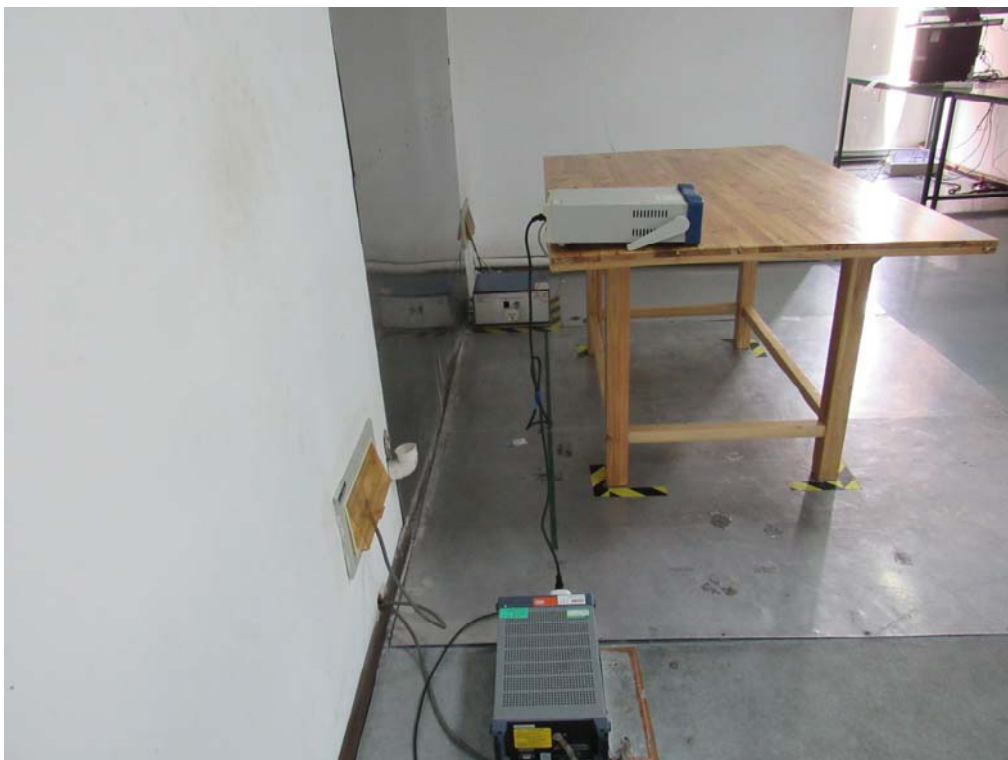
Conducted Emissions Setup Side View
