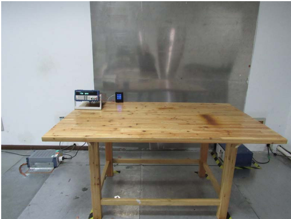
Conducted Emissions Setup Front View
