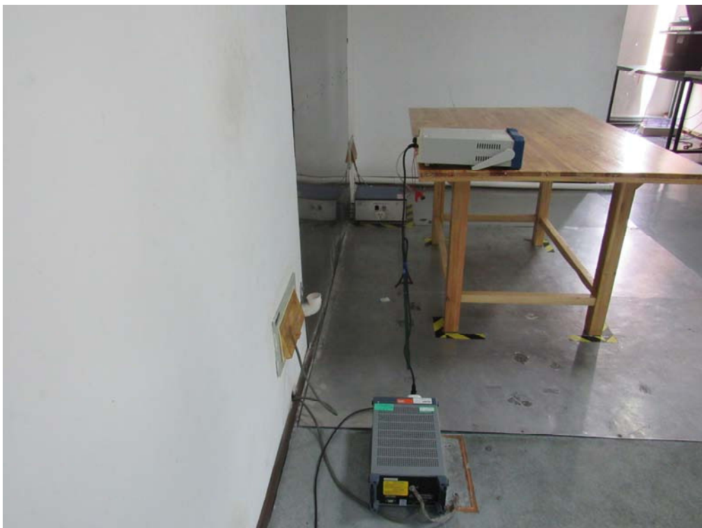
Conducted Emissions Setup Side View
