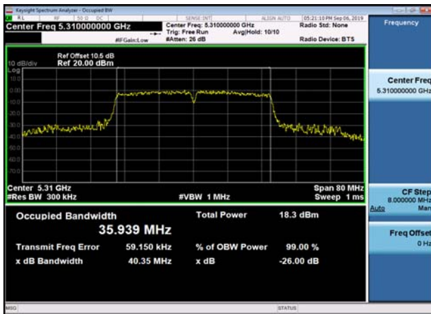
U-NII-2a 26dB Bandwidth-802.11a(20MHz )5300MHz
