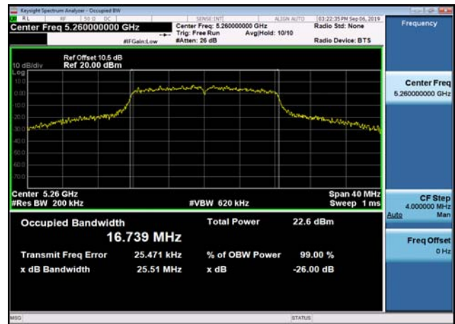
U-NII-2a 26dB Bandwidth-802.11a(20MHz )5320MHz
