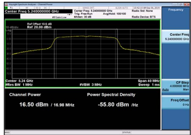
U-NII-1 Output Power-802.11a(20MHz) ,5240MHz
