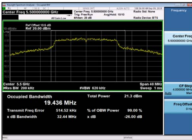
U-NII-2c 26dB Bandwidth-802.11a(20MHz) ,5500MHz
