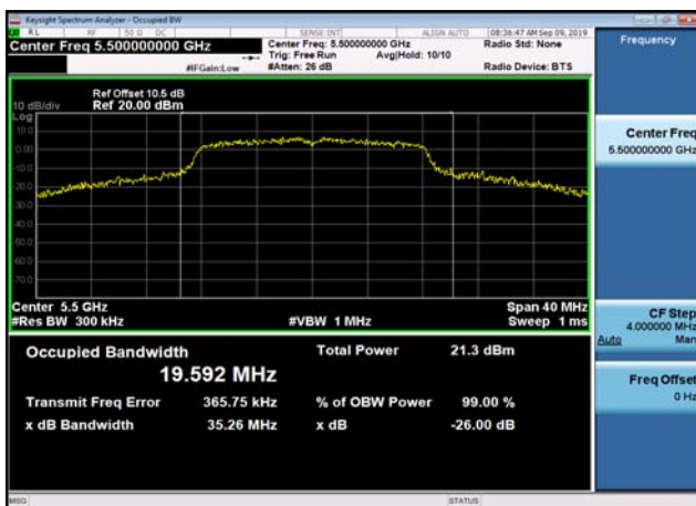
U-NII-2c 99% Bandwidth-802.11a(20MHz) ,5500MHz
