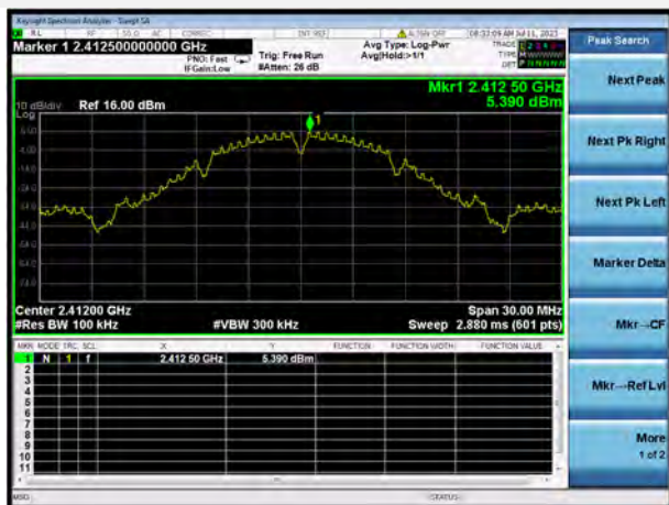
802.11b LOW CHANNEL, CARRIER LEVEL
