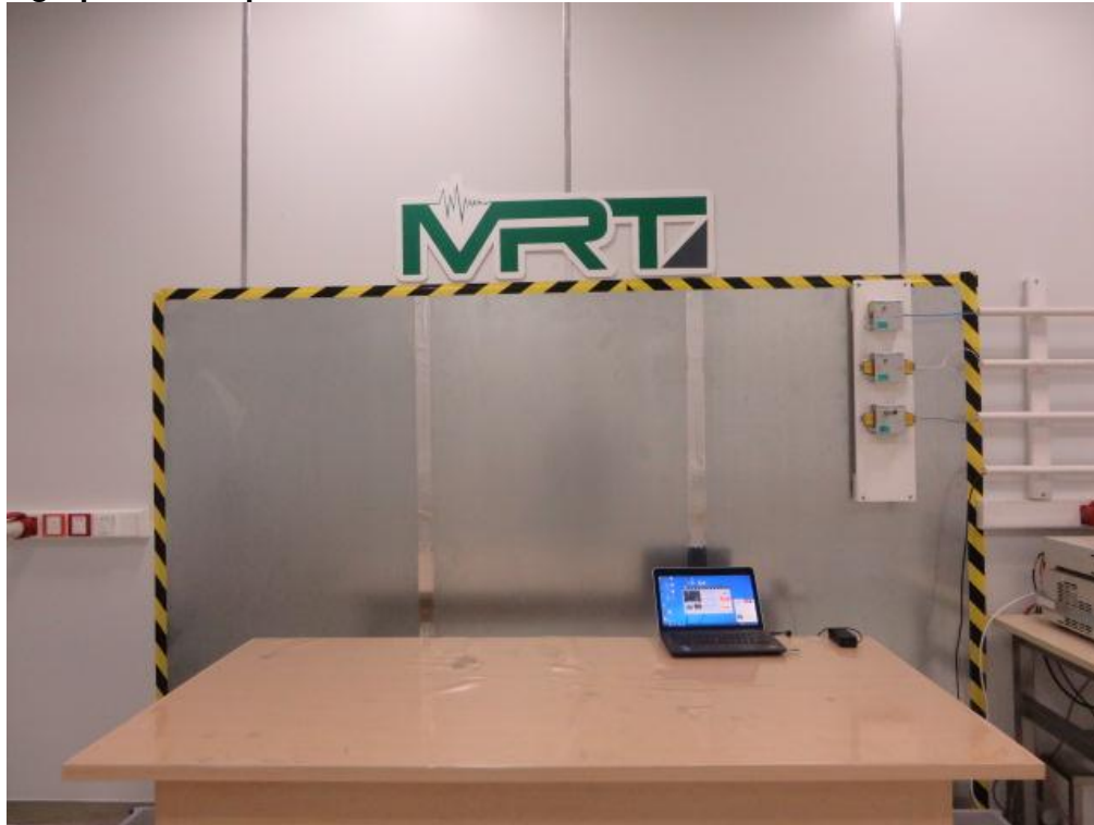
Photograph 1: Set-up for Conducted Emissions
