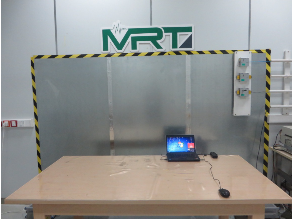
Photograph 4: Set-up for Conducted Emission Test
