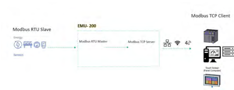
Figure 3-22: Modbus RTU to Modbus TCP
