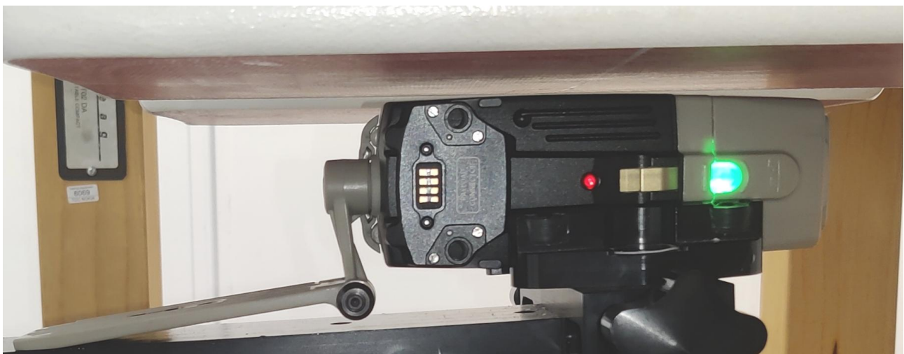
Figure 9 Right side of the device with 5mm separation against the phantom.
