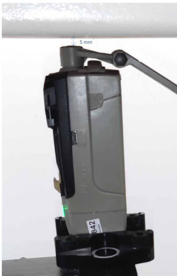
Figure 10 Back side of the device with 5mm separation against the phantom
