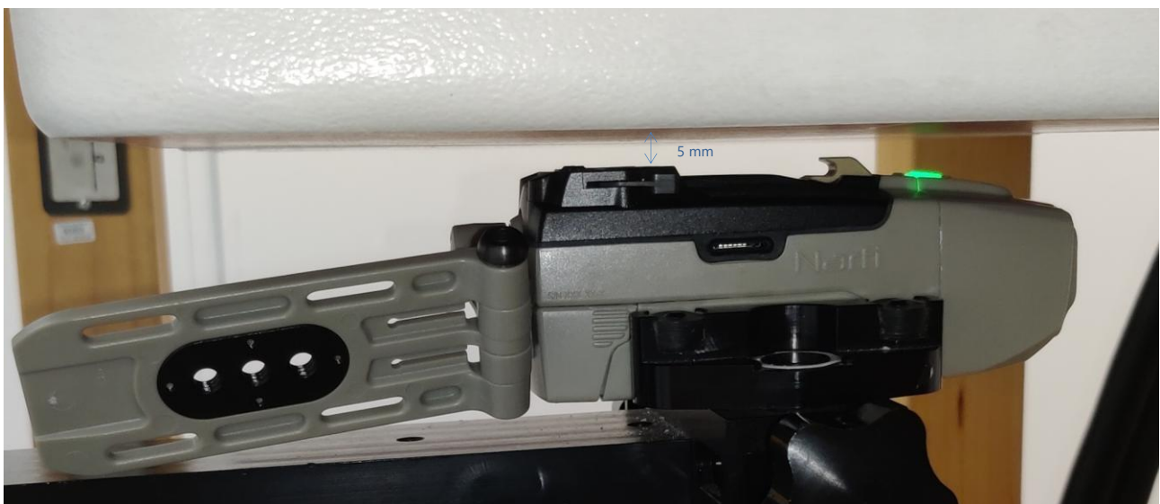
Figure 7 Bottom side of the device with 5mm separation against the phantom.
