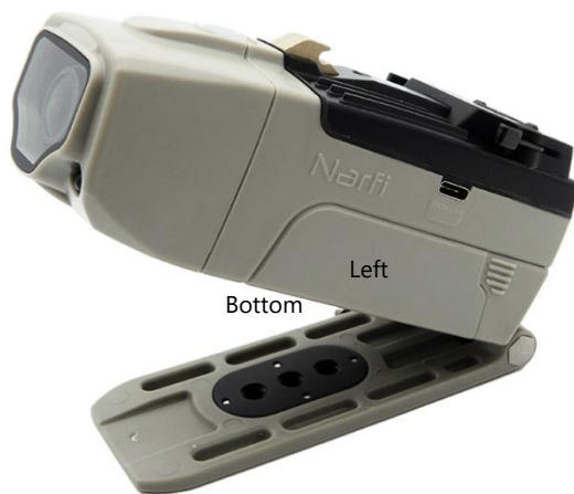
Figure 5 Photo of the DUT, device has a swivel plane at the bottom that the pole can attach to.
