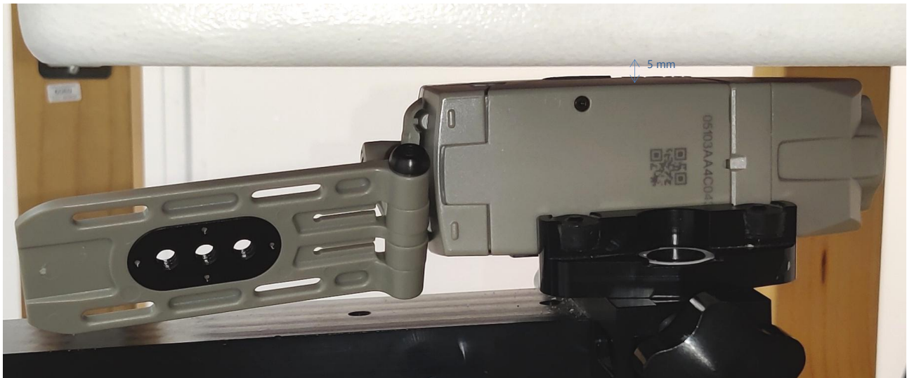
Figure 8 Left side of the device with 5mm separation against the phantom.
