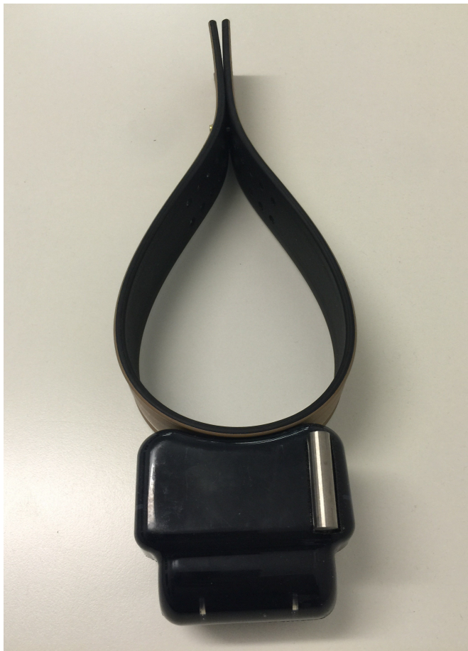
Figure 1: VERTEX PLUS Survey collar with magnet attached
