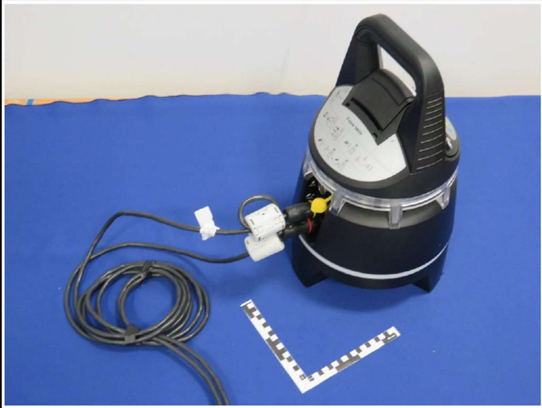
EUT WITH RS485 CABLES IN PERSPECTIVE
