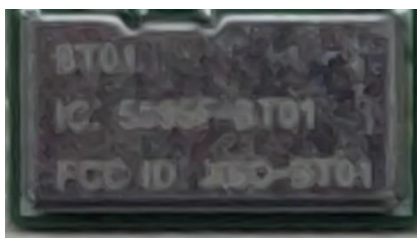
Figure 10.1-1 - picture of BT01 Shield can with laser marking
