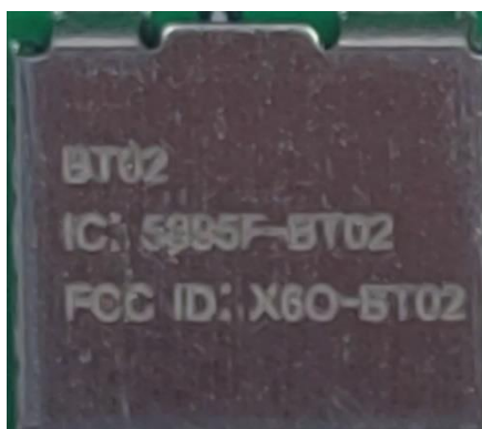
Figure 10.1-3 -picture of BT02 Shield can with laser marking
