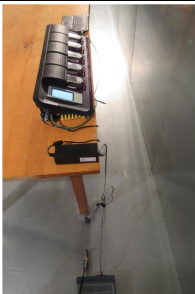
TEST SETUP EUT CONFIGURATION 2 CONDUCTED EMISSION
