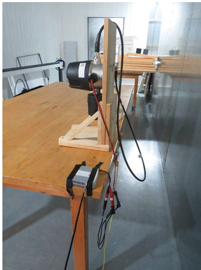
EUT 1 cable configuration
