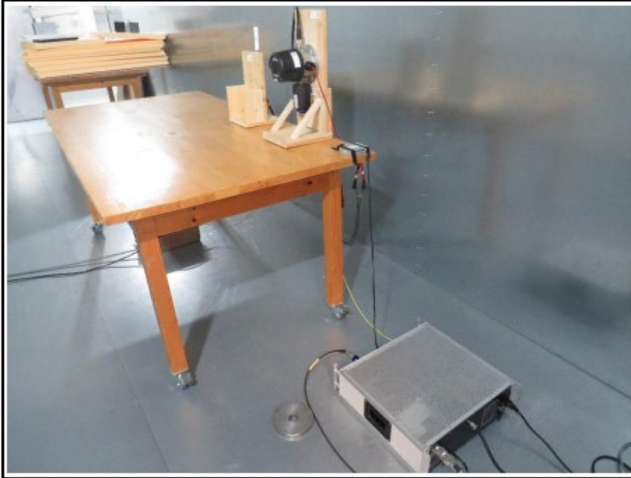
Setup for measurement 150 kHz – 30 MHz
