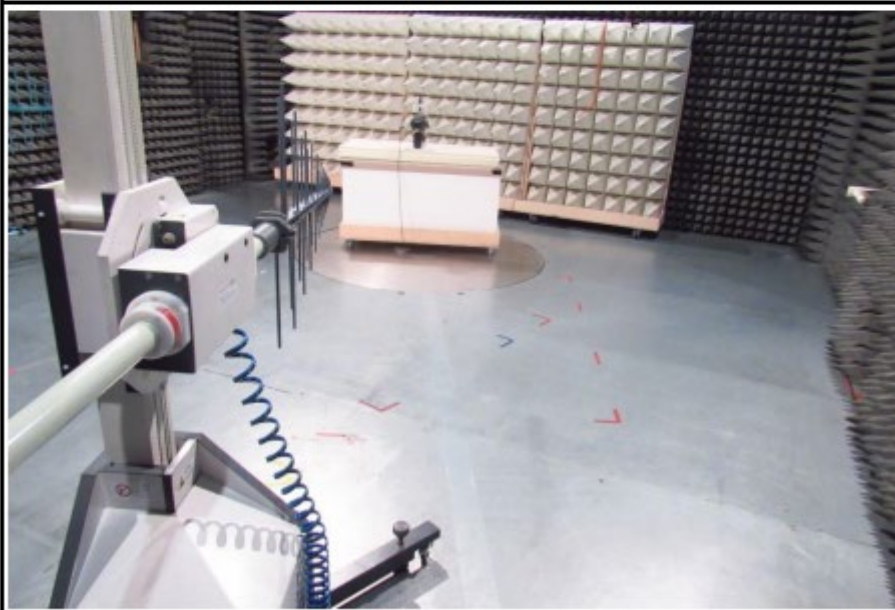
Setup for measurements below 1 GHz
