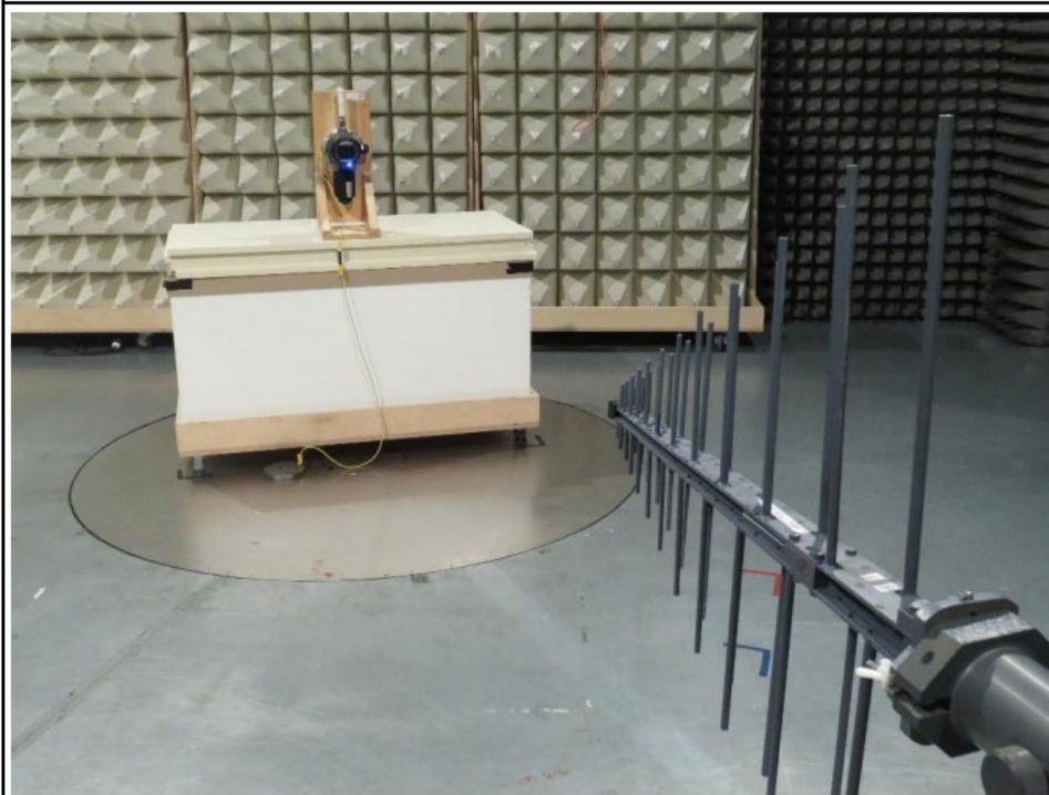
EUT 1 test setup 200 - 1000MHz vertical
