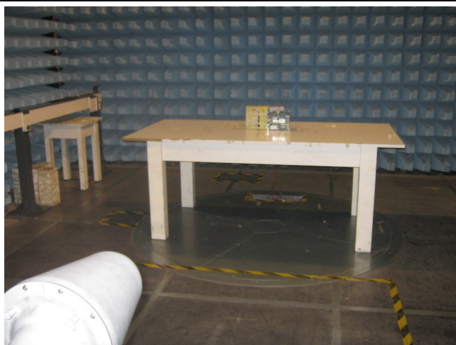
PHOTO N°5 SETUP FOR RADIATED MEASUREMENT >1GHz
