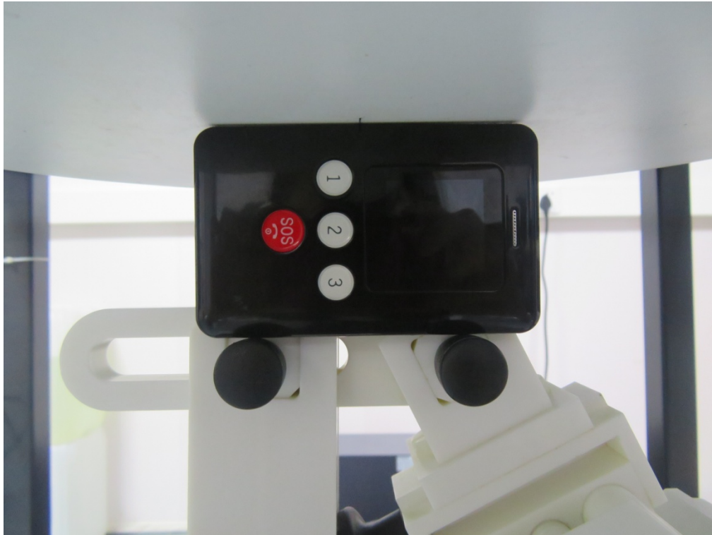
0mm body-worn Left Side Setup Photo
