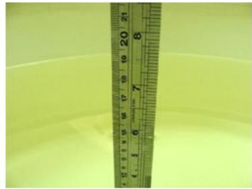
Fig 6.2 Photo of Liquid Height for Body SAR
