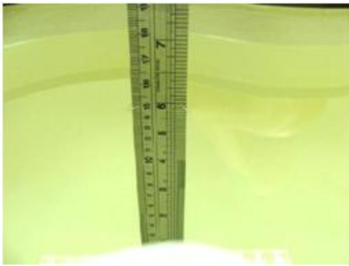
Fig 6.1 Photo of Liquid Height for Head SAR
